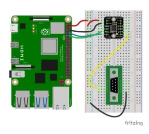
Pi 3.3V to breakout Vin (red wire)
