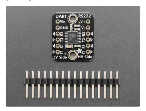
If you want to use a microcontroller or microcomputer to chat with a RS-232 then thankfully all you need is a serial port / UART (something just about any microcontroller has) and a level shifter. The level shifter is required because while most UARTs are 0-3.3V or 0-5V logic level, RS-232 requires +-6 to +-10V, yep the signal voltage goes negative! That means a specialized shifter is required, one that can generate the extra high and low voltages and also safely convert the logic levels.
