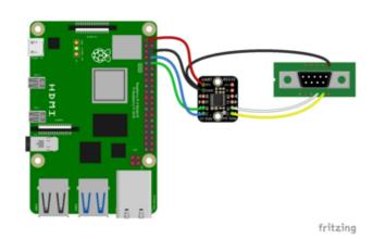
Pi 3.3V to breakout Vin (red wire)
