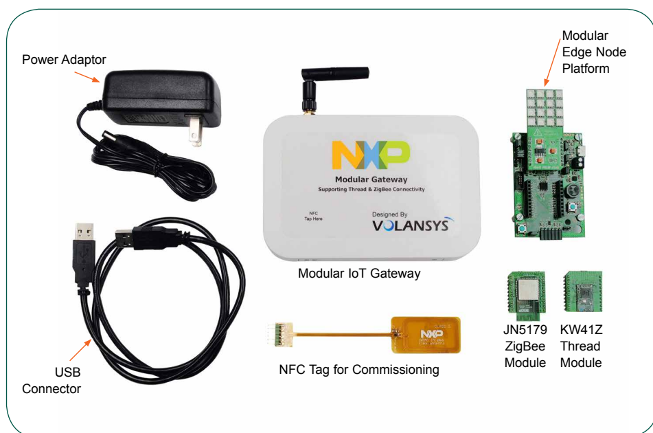
FIGURE 1: SLN-IOT-GPI: IDEX FOR GENERAL PURPOSE IOT SYSTEMS
