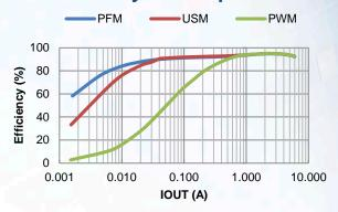
VIN = 12V, VOUT = 5V,  $L = 1.5\mu H$ ,  $f_{SW} = 800kHz$
