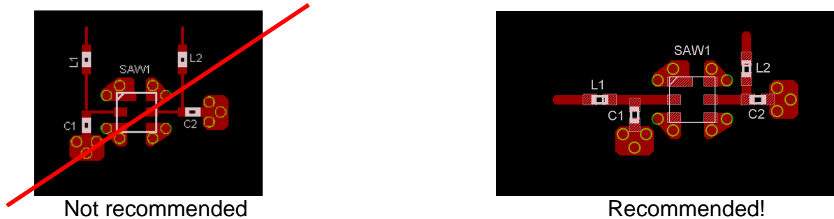
Figure 4A and Figure 4B: Not recommended and recommended placement of inductors
